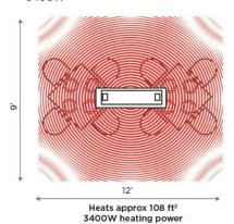
\*Heat area dependent on ambient temperature and wind. Optimum conditions experienced at approx 15.5°C/60°F & in a low wind covered environment .
